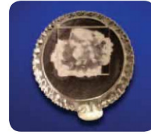
• After 300 cycles: Thermal grease voids and pumps out
